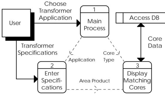
Figure 2: Data flow diagram of core selection process.
