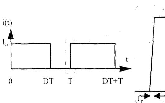
Fig. 1: Pulsed current waveform with a duty-cycle of  $D$  and a rise time  $t_r$ .
