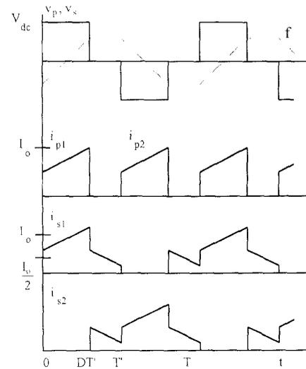
Fig. 5: Push-pull converter, waveforms.
