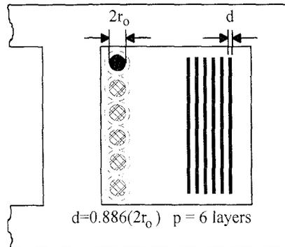
Fig. 2: Equivalent layers in a wire wound winding.
