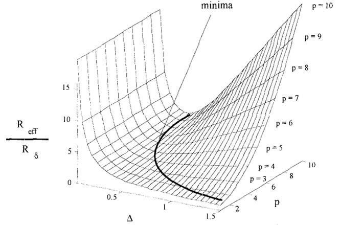
Fig. 3: Plot of  $R_{\text{eff}}/R_{\delta}$  versus  $\Delta$ , for  $N = 13$  harmonics,  $D = 50\%$  duty-cycle.
