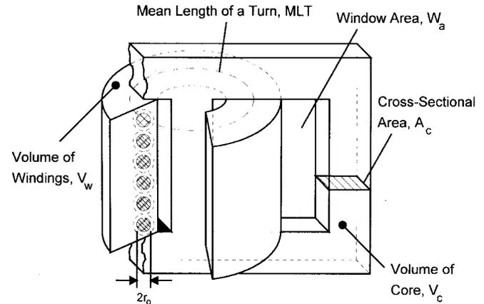
Fig. 1. Typical layout of a transformer.
