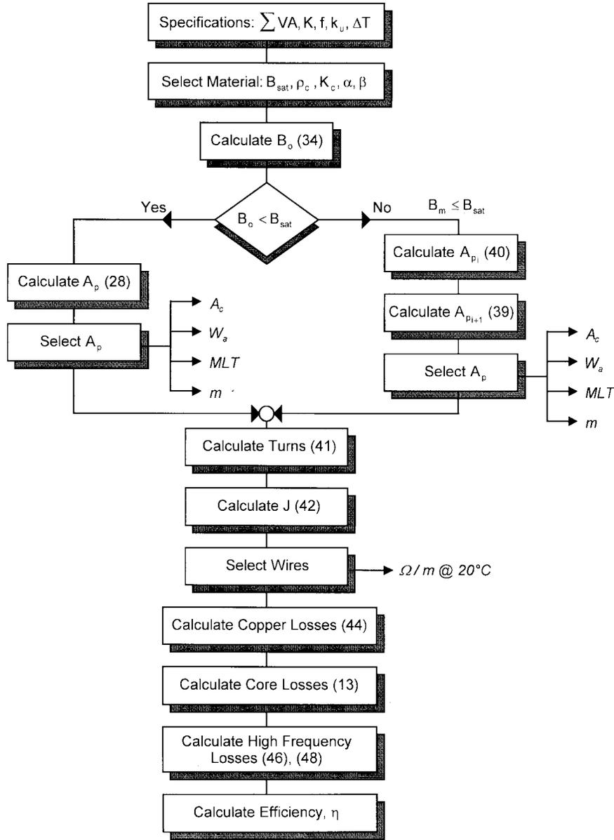
Fig. 3. Flowchart of design process.
