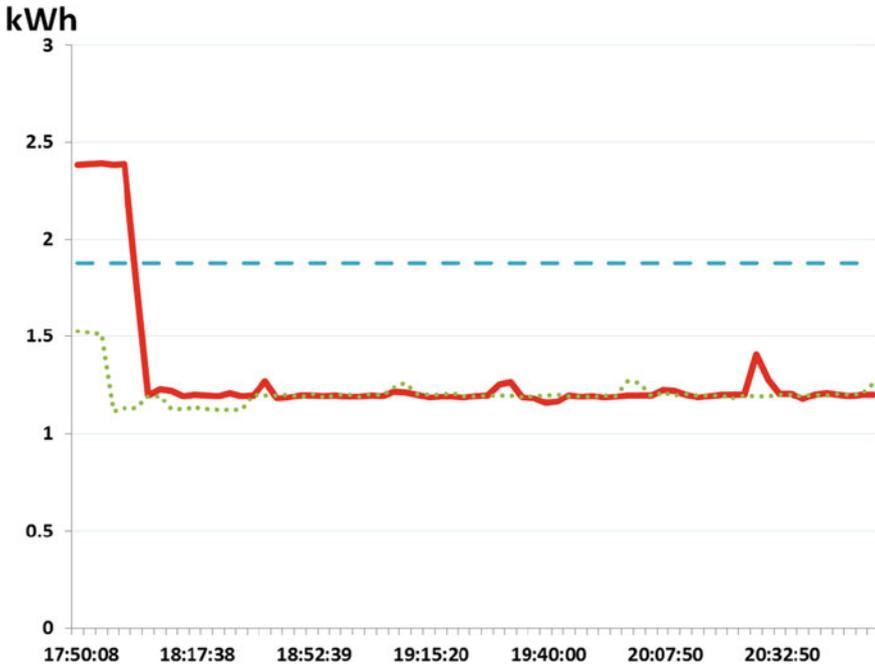
**Fig. 9** Energy usage comparison—*dashed line* is average energy usage from control period, the *solid line* is energy usage with actuation, and the *dotted line* is a day when devices were turned off manually
