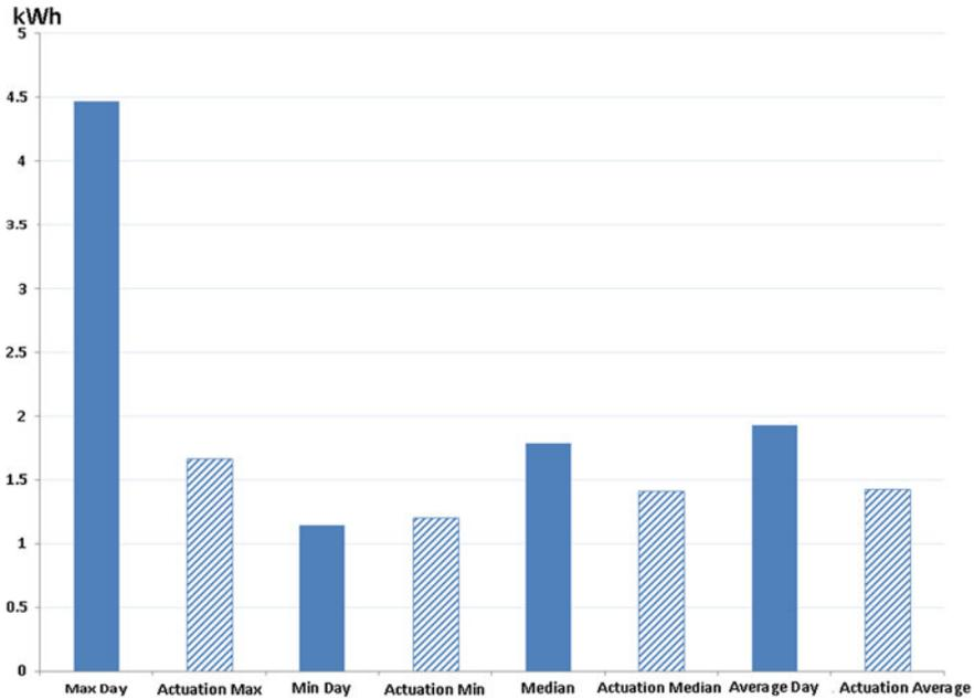
**Fig. 8** Daily energy usage—average, max, min, median of control period and actuation period
