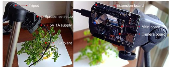
**Figure 3: Real-world testing: Inference on Sony Spresense.**
